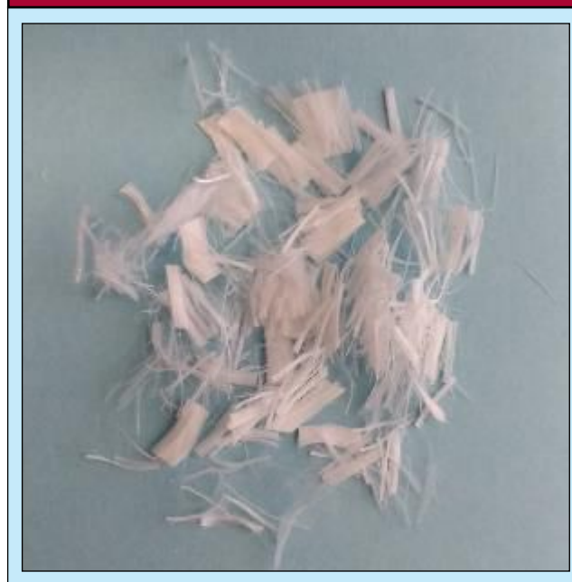
Figure 2 - staple fibers are typically longer than 6 mm
