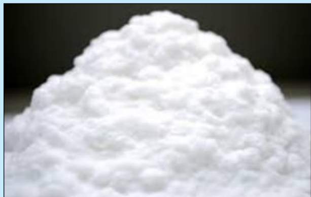
Figure 1 - flock is a short cut fiber, usually less than 6 mm
