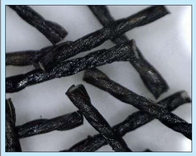
Figure 4 - fiber cord is a constructed fiber bundle
