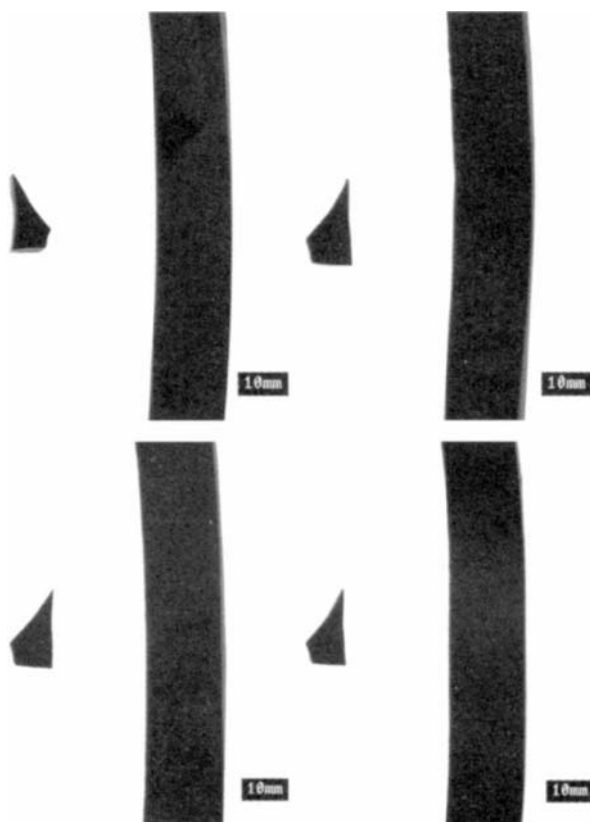
Figure 17.4 Photographs of Garvey die extrudate [8].
