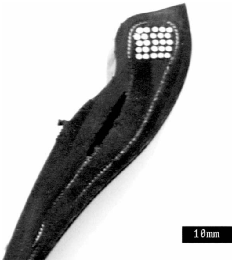
Figure 15.9 Failure deep within chafer/bead region after high speed testing.
