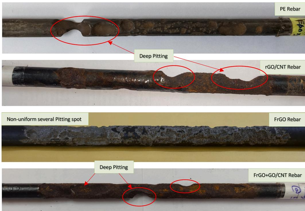
Fig. 21. Corroded rebars with different coatings.
