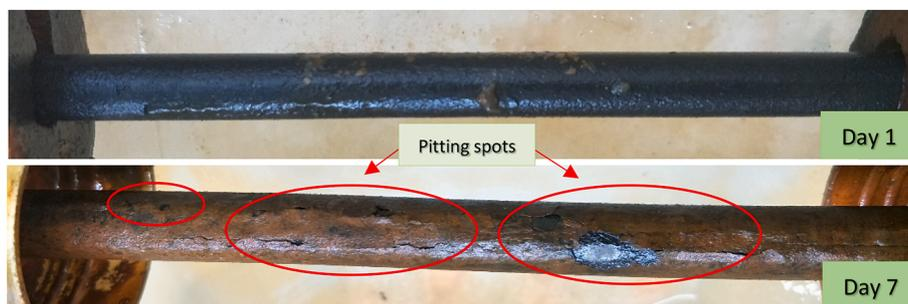
Fig. 7. Visual images of control (uncoated) rebars.
