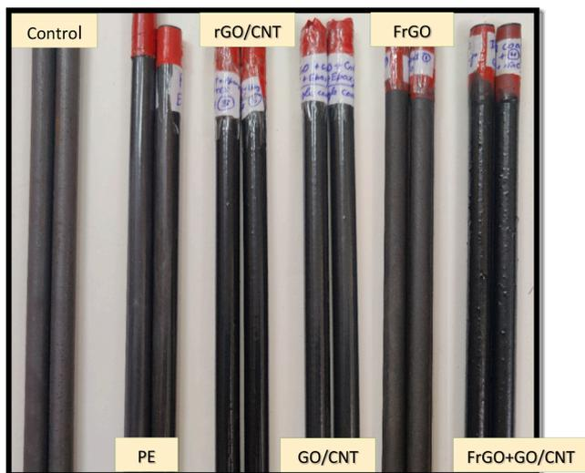
Fig. 2. Control bar and prepared coated bars.
