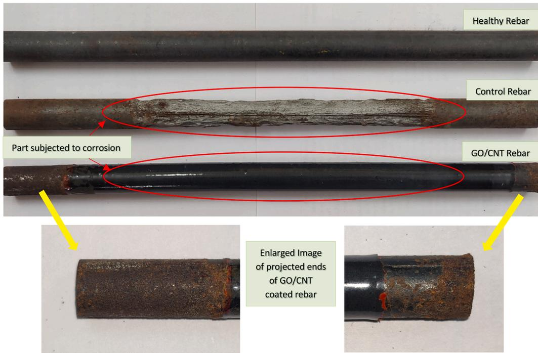
Fig. 20. Condition of healthy rebar, corroded control rebar and GO/CNT coated rebar.
