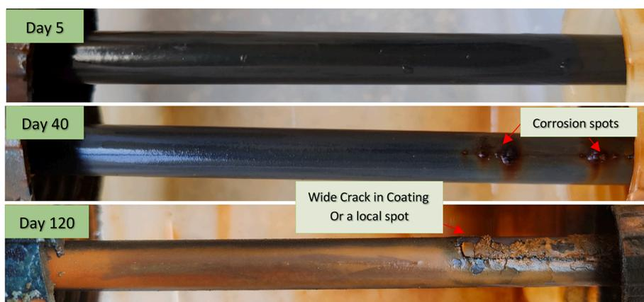
Fig. 9. Visual images of rGO/CNT coated rebar.
