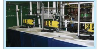
1,000 microsiemens per centimeter ( $\mu$ S/cm) to maintain an acceptable level of water discharge and replacement. The water baths include sprays that contact the rubber as it comes out of the extruder, and then the section where the rubber is submerged in the bath water for further cooling.
