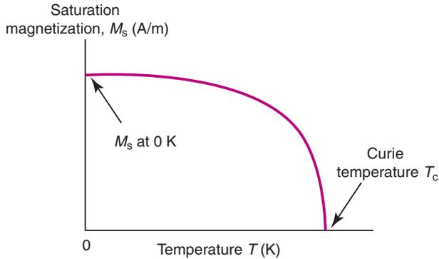
Figure 15.4 Saturation magnetization decreases with temperature, falling to zero at the Curie temperature,  $T_c$ .
