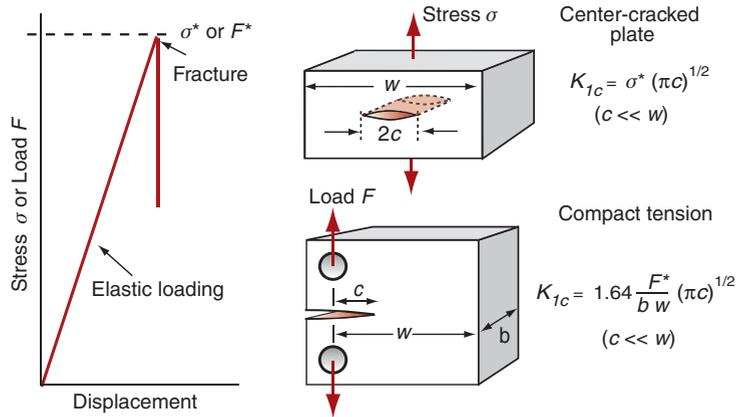
Figure 8.4 Measuring fracture toughness,  $K_{1c}$ . Two test configurations are shown here; others are described in Chapter 10.
