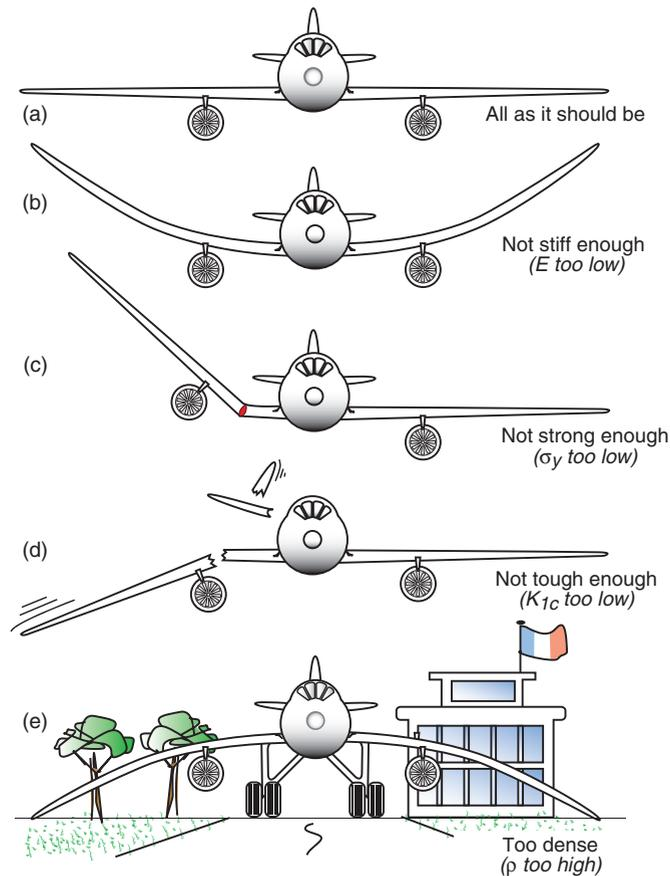
Figure 1.2 Mechanical properties.
