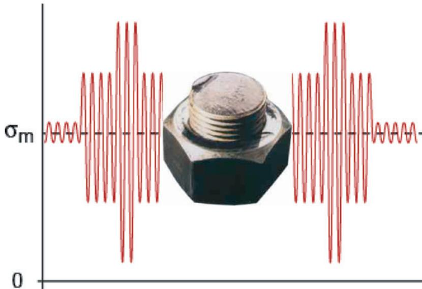
A bolt that has failed by fatigue. The fatigue crack initiated at the root of a thread, which acts as a notch, concentrating stress. (Image courtesy Bolt Science ([www.Boltscience.com](http://www.Boltscience.com)))
