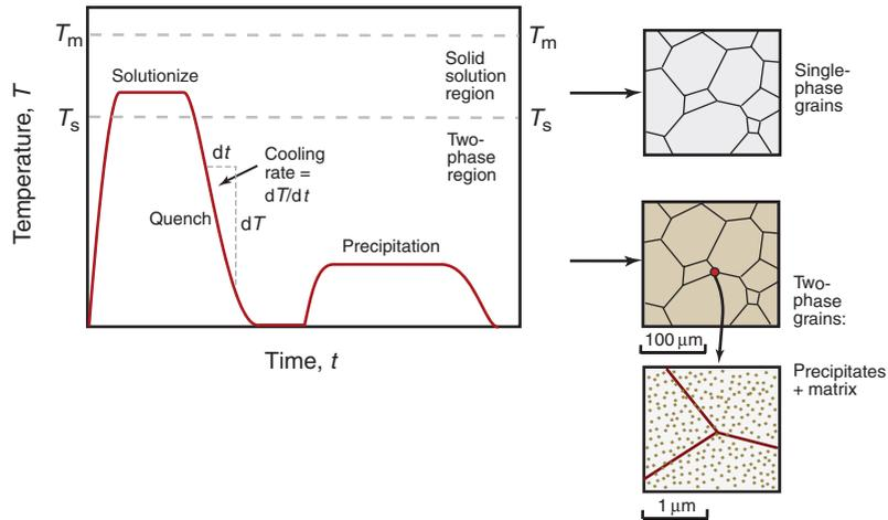
**Figure 19.7** Schematic thermal profile for heat treatments that produce precipitation hardening, illustrating microstructural changes being induced: a solid solution at high temperature and precipitation of hardening particles (shown on an enlarged scale) at a lower temperature.
