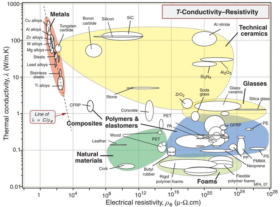
Figure 14.5 Electrical resistivity  $\rho_e$  and thermal conductivity  $\lambda$ .
