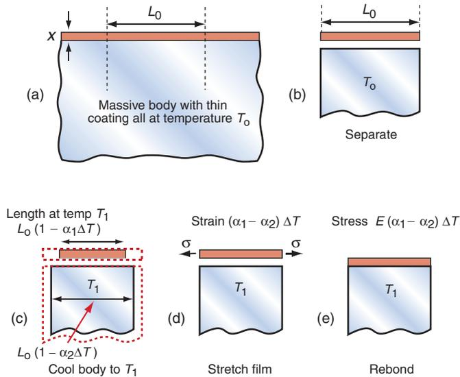
**Figure 12.12** Thermal stresses in thin films arise on cooling or heating when their expansion coefficients differ. Here that of the film is  $\alpha_1$  and that of the substrate, a massive body, is  $\alpha_2$ .
