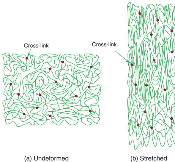
**Figure 4.20** The stretching of an elastomer. Here the structure has been stretched to twice its original length. The stretching causes alignment, producing crystal-like regions. Thermal vibration drives the structure back to the one on the left, restoring its shape.
