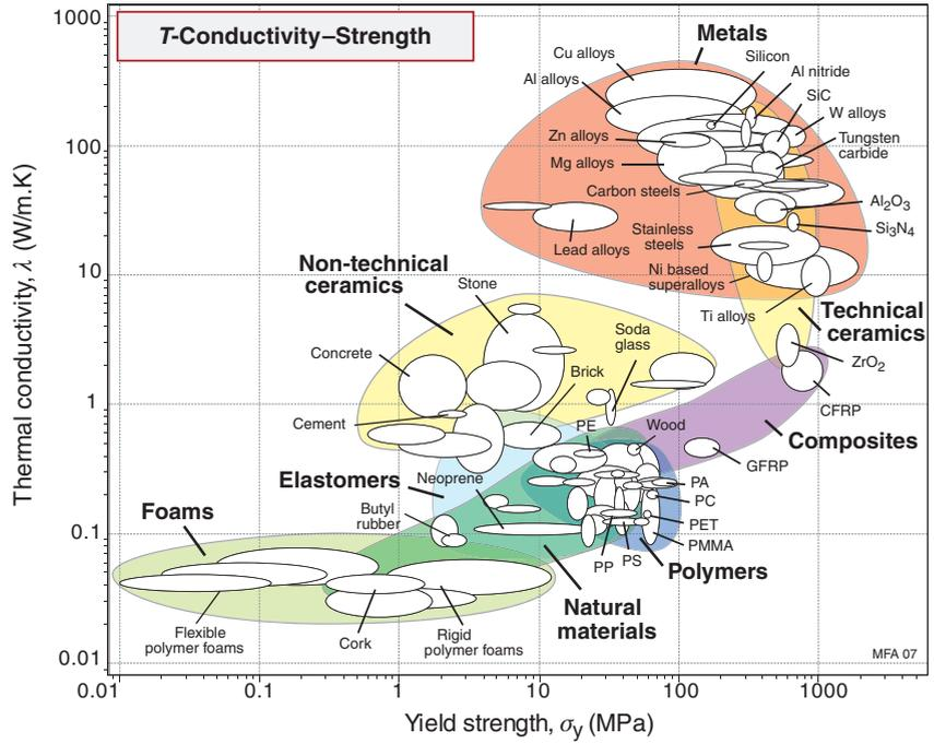
Figure 12.6 Thermal conductivity  $\lambda$  and strength  $\sigma_y$ .
