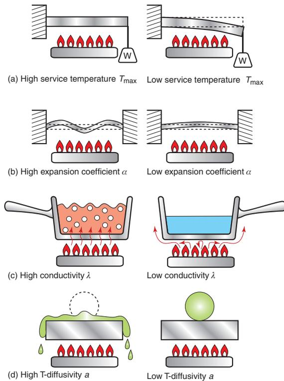
Figure 1.3 Thermal properties.
