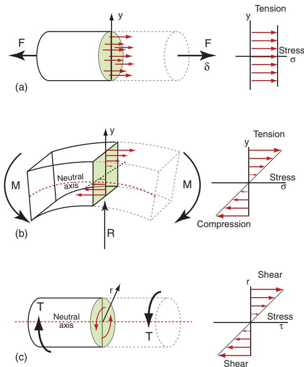
**Figure 5.1** (a) A tie with a cross-section  $A$  loaded in tension. Its stiffness is  $S = F/\delta$ . (b) A beam of rectangular cross-section loaded in bending. The stress  $\sigma$  varies linearly from tension to compression, changing sign at the neutral axis, resulting in a bending moment  $M$ . (c) A shaft of circular cross-section loaded in torsion.
