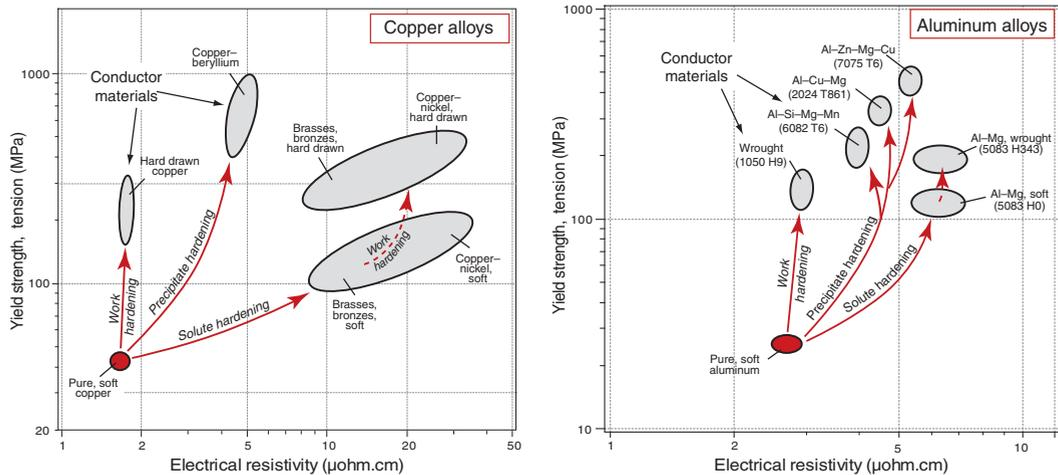
**Figure 14.11** The best choice of material for a cable is one with high strength and low resistivity, but strengthening mechanisms increase resistivity. Work hardening and precipitation hardening do so less than solute hardening.
