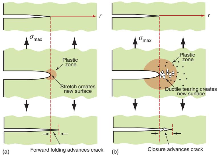
**Figure 9.9** (a) In high-cycle fatigue a tiny zone of plasticity forms at the crack tip on each tension cycle; on compression the newly formed surface folds forwards. (b) In low-cycle fatigue the plastic zone is large enough for voids to nucleate and grow within it. Their coalescence further advances the crack.
