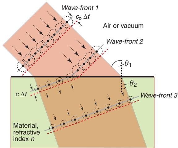
**Figure 16.4** The Fresnel construction, explaining why a light beam is bent on entering a material of higher refractive index.
