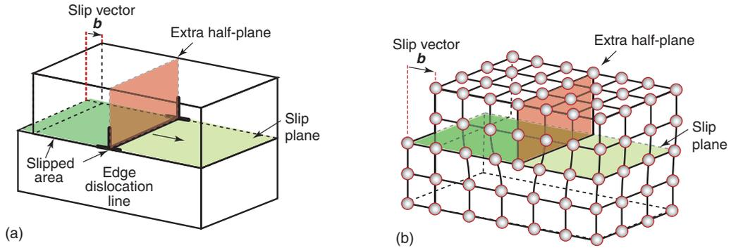
**Figure 6.11** (a) Making a dislocation by cutting, slipping and rejoining bonds across a slip plane. (b) The atom configuration at an edge dislocation in a simple cubic crystal. The configurations in other crystal structures are more complex but the principle remains the same.
