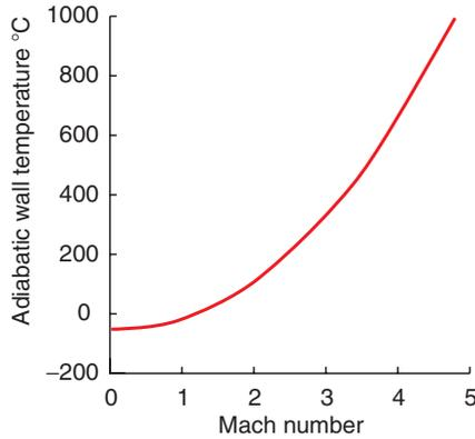
**Figure 13.24** Adiabatic heating as a function of speed.
