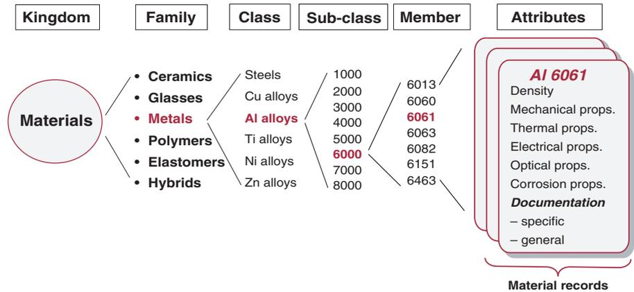
Figure 2.3 The taxonomy of the kingdom of materials and their attributes. Computer-based selection software stores data in a hierarchical structure like this.
