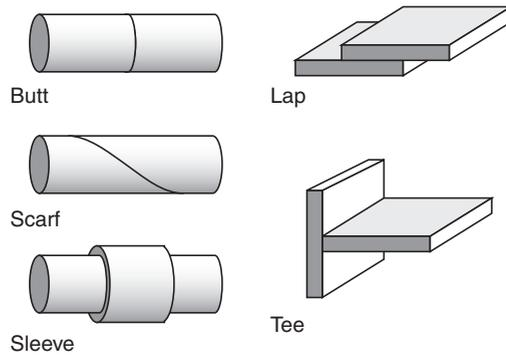
Figure 18.13 Joint geometries.
