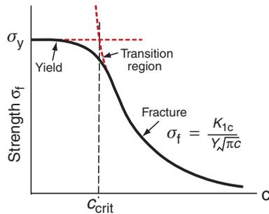
Figure 8.7 The transition from yield to fracture at the critical crack length  $c_{crit}$ .
