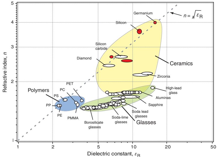
**Figure 16.5** A chart of refractive index and dielectric constant, showing the approximate relationship  $n = \sqrt{\epsilon_R}$ . (This chart and the next were made using Level 3 of the CES database.)
