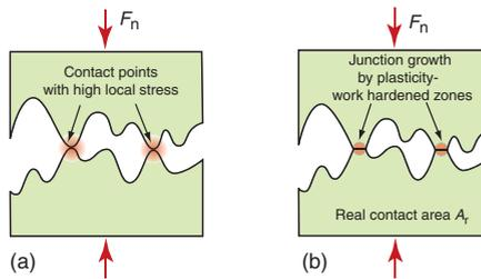
**Figure 11.5** When surfaces first touch, high contact stresses appear, as in (a). These cause plasticity and junction growth until the junction area  $A_r$  can just support the load  $F_n$  without further plasticity, as in (b).
