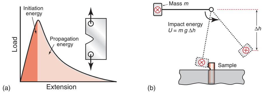
Figure 8.2 (a) The tear test. (b) The impact test. Both are used as acceptance tests and for quality control, but neither measures a true material property.
