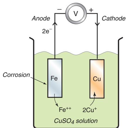
Figure 17.8 A bi-metal corrosion cell. The corrosion potential is the potential to which the metal falls relative to a hydrogen standard.
