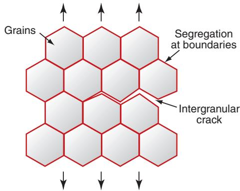
Figure 8.14 Chemical segregation can cause brittle intergranular cracking.
