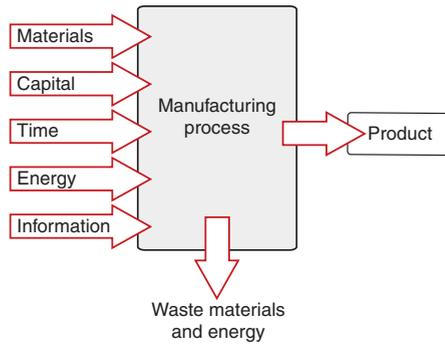
Figure 18.15 The inputs to a manufacturing process.
