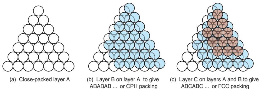
**Figure 4.8** (a) A close-packed layer of spheres, layer A; atoms often behave as if hard and spherical. (b) A second layer, B, nesting in the first; repeating this sequence gives ABAB . . . or CPH stacking. (c) A third layer, C, can be nested so that it does not lie above A or B; if repeated this gives ABCABC . . . or FCC stacking.
