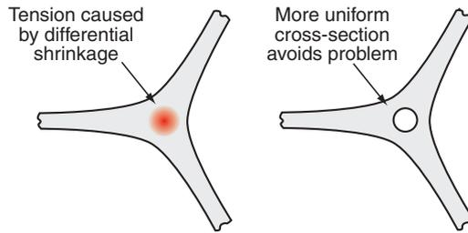
**Figure 18.6** (a) Differential shrinkage causes internal stress, distortion and cavitation in thick sections or at changes of section. (b) Good design keeps section thickness as uniform as possible, avoiding the problem.
