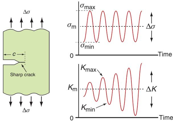
Figure 9.6 Cyclic loading of a cracked component. A constant stress amplitude  $\Delta\sigma$  gives an increasing amplitude of stress intensity,  $\Delta K = \Delta\sigma\sqrt{\pi c}$  as the crack grows in length.
