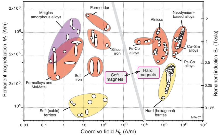
**Figure 15.8** Remanent magnetization and coercive force. Soft magnetic materials lie on the left, hard magnetic materials on the right. The red and purple envelopes enclose electrically conducting materials, the yellow ones enclose insulators.
