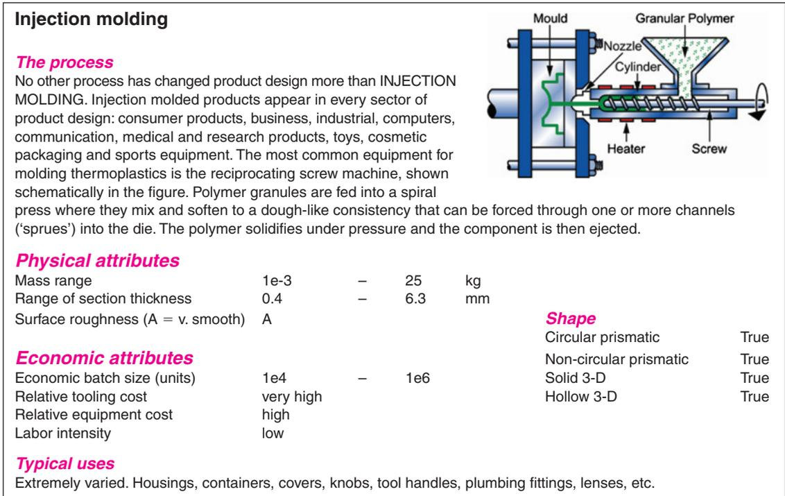
**Figure 2.11** Part of a record for a process, injection molding. The image shows how it works, and the numeric and Boolean data and text document its attributes.
