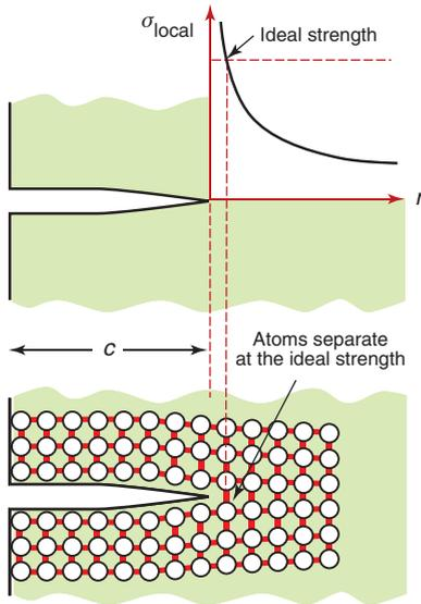
**Figure 8.11** Cleavage fracture. The local stress rises as  $1/\sqrt{r}$  towards the crack tip. If it exceeds that required to break inter-atomic bonds (the 'ideal strength') they separate, giving a cleavage fracture. Very little energy is absorbed.
