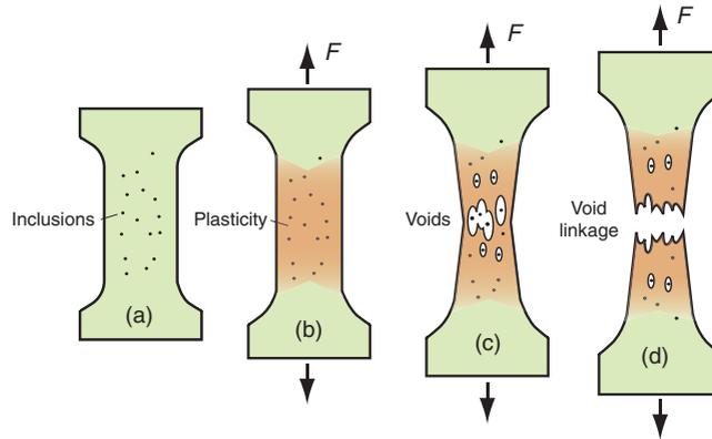
**Figure 8.12** Ductile fracture. Plasticity, shown in red, concentrates stress on inclusions that fracture or separate from the matrix, nucleating voids that grow and link, ultimately causing fracture.
