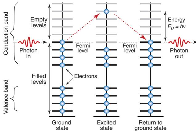
**Figure 16.8** Metals absorb photons, capturing their energy by promoting an electron from the filled part of the conduction band into a higher, empty level. When the electron falls back, a photon is re-emitted.
