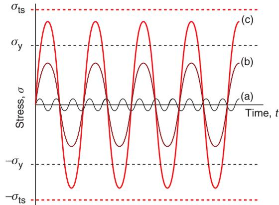
**Figure 9.1** Cyclic loading. (a) Very low amplitude acoustic vibration. (b) High-cycle fatigue: cycling well below general yield,  $\sigma_y$ . (c) Low cycle fatigue: cycling above general yield (but below the tensile strength  $\sigma_{ts}$ ).
