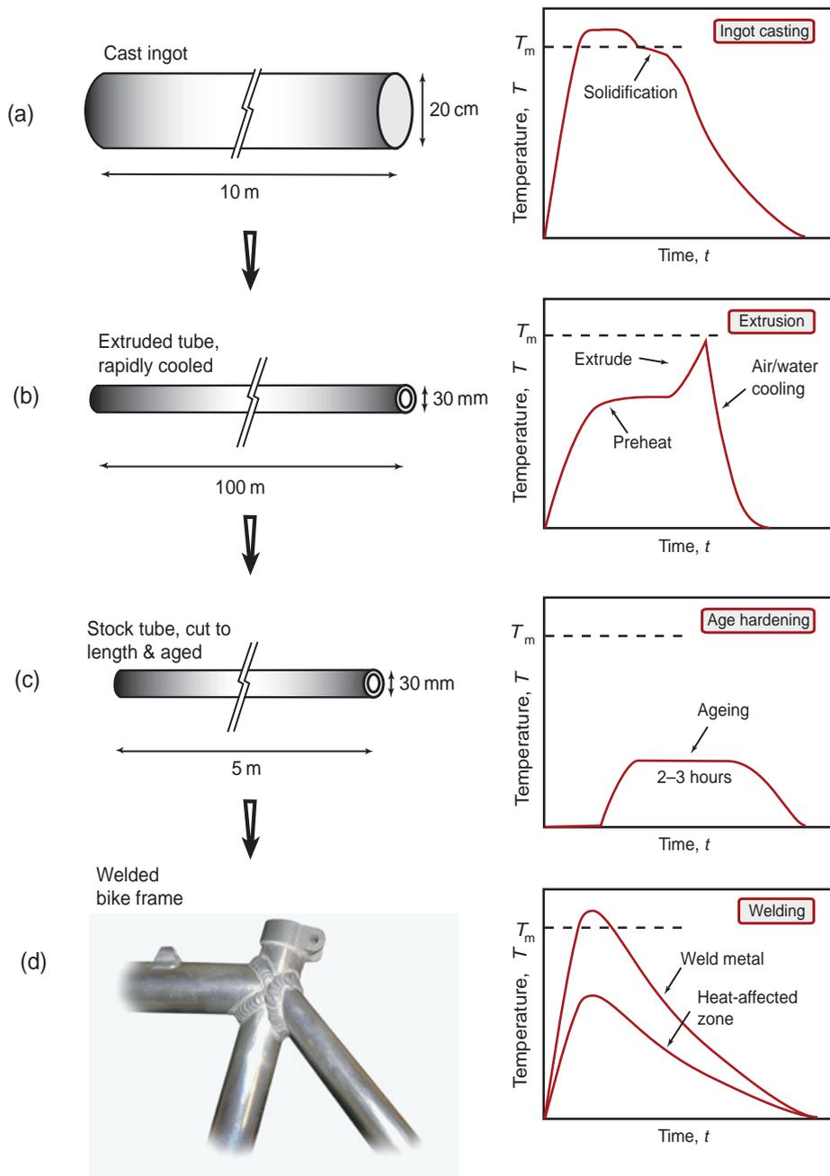
**Figure 19.11** A schematic process history for the manufacture of a bike frame in heat-treatable aluminum alloy. (a) Casting of large ingot, cut into billets for extrusion. (b) Hot extrusion into tube, incorporating the solution heat treatment and quench. (c) Sections cut to length and age hardened. (d) Assembly into the frame by arc welding.
