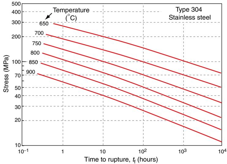
Figure 13.20 Stress-rupture time data for Type 304 stainless steel.
