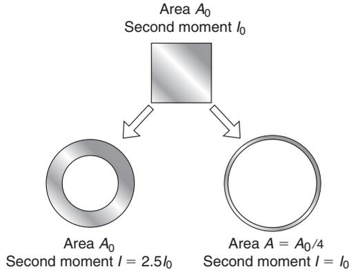
**Figure 5.8** The effect of section shape on bending stiffness  $EI$ : a square-section beam compared, left, with a tube of the same area (but 2.5 times stiffer) and, right, a tube with the same stiffness (but four times lighter).
