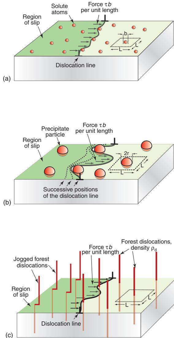
**Figure 6.18** (a) Solution hardening. (b) Precipitation or dispersion hardening. (c) Forest hardening (work hardening).
