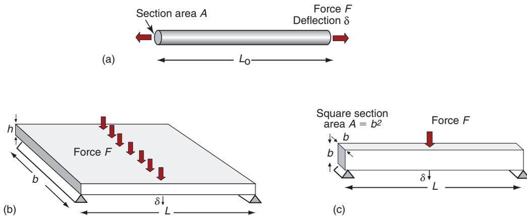
**Figure 5.7** (a) A tie with cross-section area  $A$ , loaded in tension. Its stiffness is  $S = F/\delta$  where  $F$  is the load and  $\delta$  is the extension. (b) A panel loaded in bending. Its stiffness is  $S = F/\delta$ , where  $F$  is the total load and  $\delta$  is the bending deflection. (c) A beam of square section, loaded in bending. Its stiffness is  $S = F/\delta$ , where  $F$  is the load and  $\delta$  is the bending deflection.
