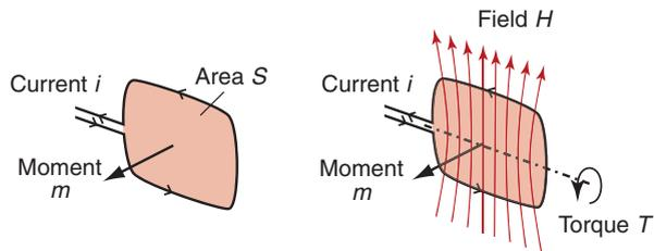
Figure 15.2 Definition of magnetic moment and moment-field interaction.
