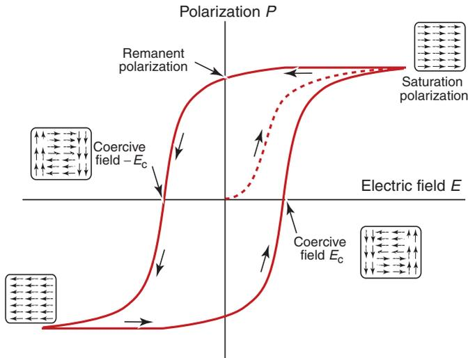
**Figure 14.18** A ferro-electric hysteresis curve.
