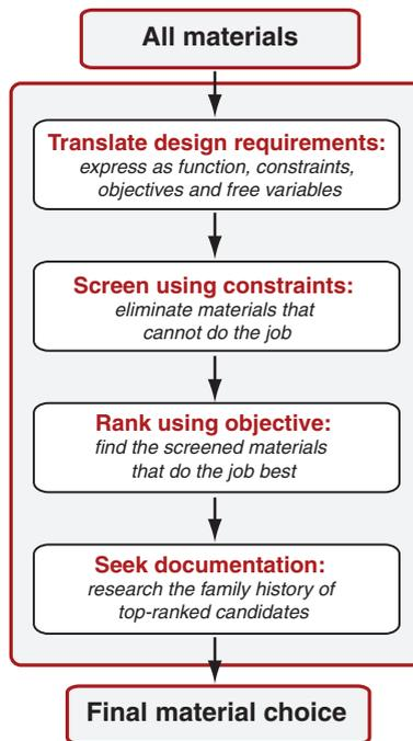
**Figure 3.6** The strategy applied to materials. The same strategy is later adapted to select processes. There are four steps: translation, screening, ranking and supporting information. All can be implemented in software, allowing large populations of materials to be investigated.
