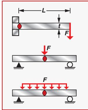
Figure 7.2 The plastic bending of beams.
