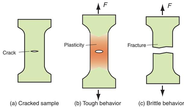
**Figure 8.1** Tough and brittle behavior. The crack in the tough material, shown in (b), does not propagate when the sample is loaded; that in the brittle material propagates without general plasticity, and thus at a stress less than the yield strength.
