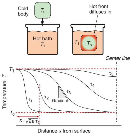
Figure 12.15 The diffusion of heat into an initially cold body.
