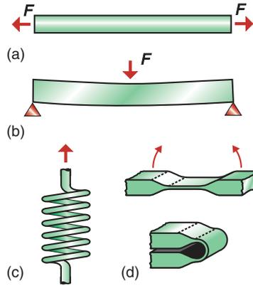
**Figure 10.3** (a, b) Load-limited design. (c) Energy-limited design. (d) Displacement-limited design. Each must perform its function without fracturing.
