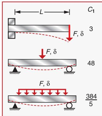
Figure 5.3 Elastic deflection of beams. The deflection  $\delta$  of a span  $L$  under a force  $F$  depends on the flexural stiffness  $EI$  of the cross-section and the way the force is distributed. The constant  $C_1$  is defined in equation (5.5).
