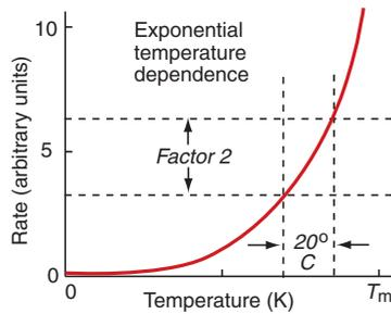
Figure 13.2 The exponential increase of rate of straining with temperature at constant load. The rate can double with a rise of temperature of only  $20^\circ\text{C}$ .
