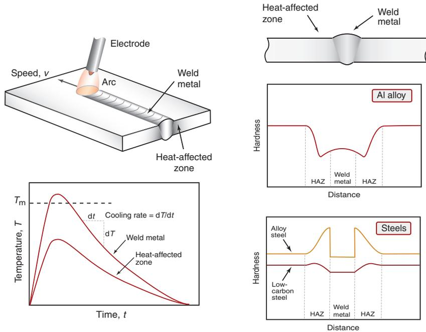
**Figure 19.9** A weld cross-section with corresponding thermal histories in the weld metal and heat-affected zone. Below are typical hardness profiles induced across welds in heat-treatable aluminum alloys, low-carbon steel and low-alloy steel.
