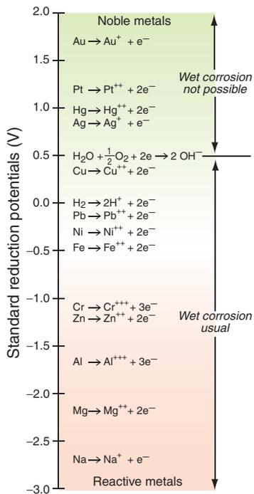
Figure 17.7 Standard reduction potentials of metals.
