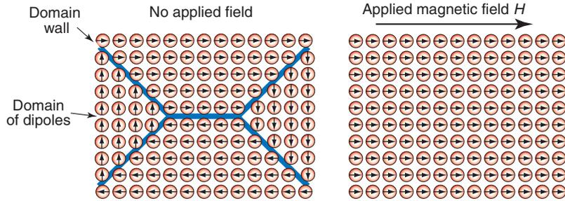
**Figure 15.13** An applied field causes domain boundaries to move. At saturation the sample has become a single domain, as on the right. Domain walls move easily in soft magnetic materials. Hard magnetic materials are alloyed to prevent their motion.
