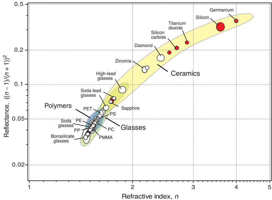
**Figure 16.6** A chart of refractive index and reflectance. The materials with open circles are transparent to visible light; those with red circles are transparent to infrared and below, but not to visible radiation. Diamond is special because of its high refractive index, reflectance and transparency in the visible spectrum.
