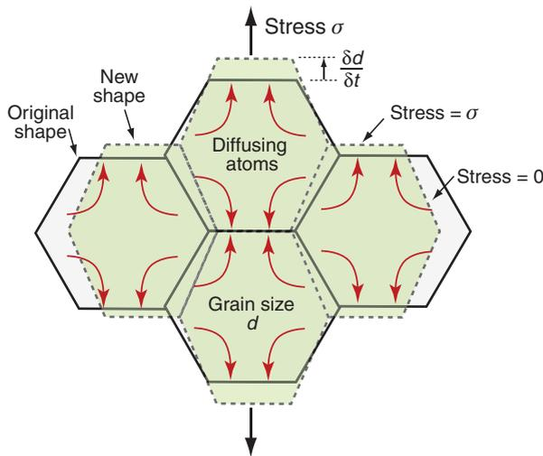
Figure 13.12 Deformation by diffusion alone, giving *diffusional flow*.
