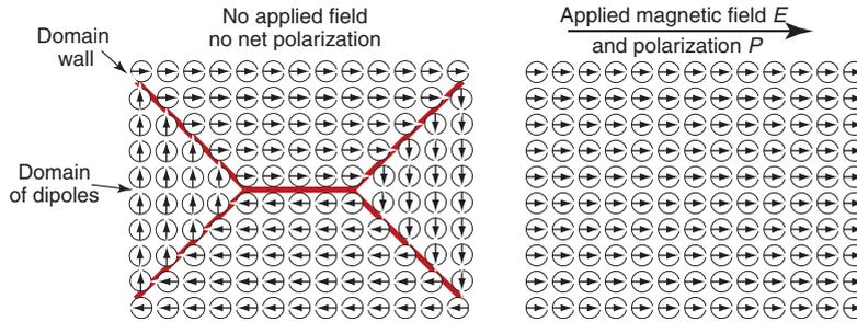
**Figure 14.17** Ferro-electric domains arrange themselves so that their dipole moments cancel. In an electric field  $E$  they align, giving the crystal a net dipole moment, which can be large.
