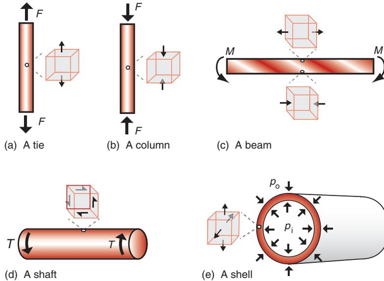
Figure 4.2 Modes of loading and states of stress.
