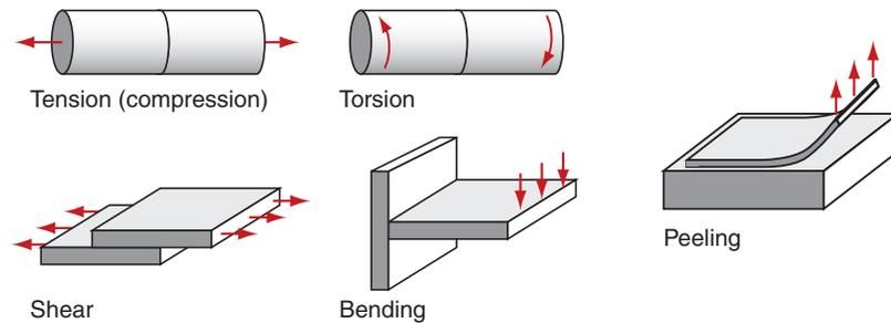
Figure 18.14 Standard modes of loading for joints.
