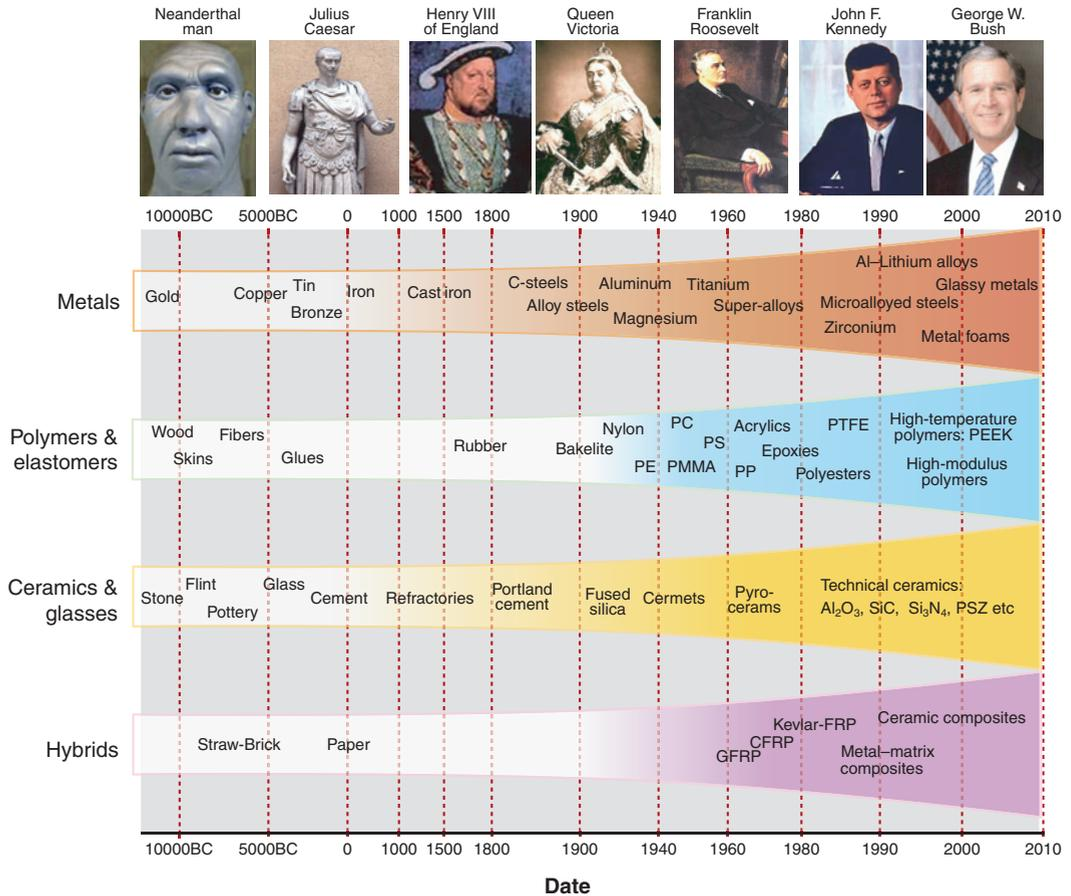
**Figure 1.1** The development of materials over time. The materials of pre-history, on the left, all occur naturally; the challenge for the engineers of that era was one of shaping them. The development of thermochemistry and (later) of polymer chemistry enabled man-made materials, shown in the colored zones. Three—stone, bronze and iron—were of such importance that the era of their dominance is named after them.
