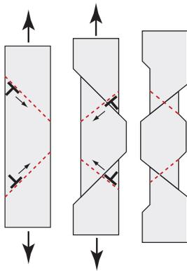
Figure 6.14 Dislocation motion causes extension
