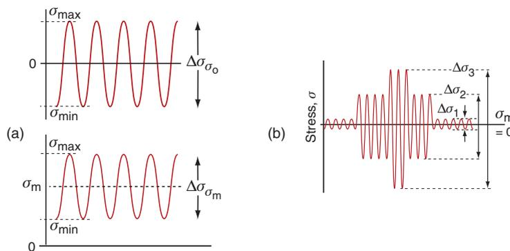
**Figure 9.5** (a) The endurance limit refers to a zero mean stress. Goodman's law scales of the stress range to a mean stress  $\sigma_m$ . (b) When the cyclic stress amplitude changes, the life is calculated using Miner's cumulative damage rule.
