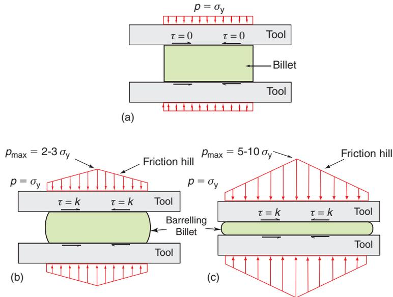
**Figure 18.7** The influence of friction and aspect ratio on open die forging. (a) Uniaxial compression with very low friction. (b) With sticking friction the contact pressure rises in a 'friction hill' causing barrelling. (c) The greater the aspect ratio, the greater the pressure rise and the barrelling.
