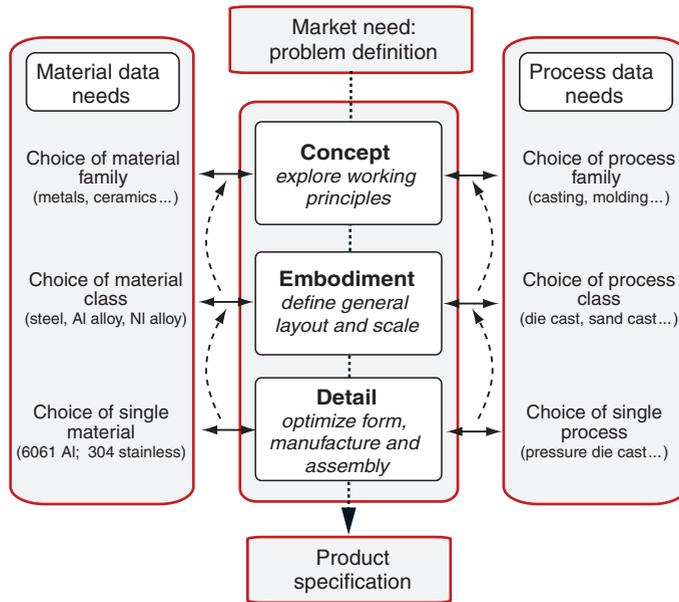
**Figure 3.1** The design flow chart, showing how material and process selection enter. Information about materials is needed at each stage, but at very different levels of breadth and precision. The broken lines suggest the iterative nature of original design and the path followed in redesign.
