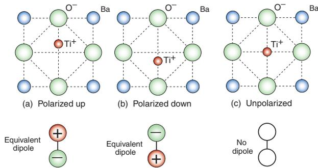
**Figure 14.16** Ferro-electric materials have a permanent dipole moment that can switch: here the  $\text{Ti}^+$  ion can flip from the upper to the lower position. Above the Curie temperature the asymmetry disappears.
