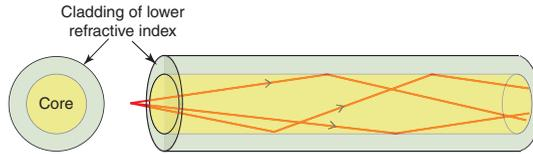
**Figure 16.12** An optical fiber. The graded refractive index traps light by total internal reflection, making it follow the fiber even when it is curved.
