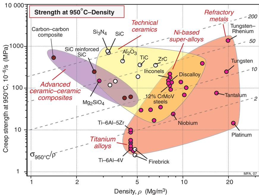
**Figure 13.8** A chart showing the strength of selected materials at a particularly high temperature—950°C and a strain rate of  $10^{-6}/\text{s}$ —plotted against density. Software allows charts like this to be constructed for any chosen temperature. (The chart was made with a specialized high-temperature materials database that runs in the CES system.)
