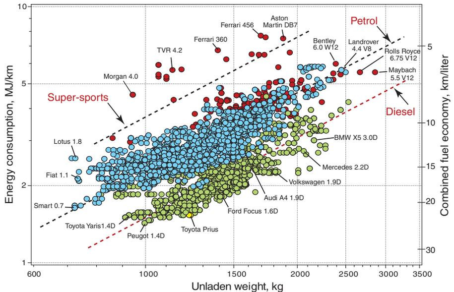
**Figure 20.13** Energy consumption and fuel economy of 2005 model European cars, plotted against the unladen weight. The open red symbols are diesels, the open black are petrol driven and the full red symbols are for cars designed with performance, above all else, in mind. The broken lines are best fits to data for each type. Note the near-linear dependence of energy consumption on weight.
