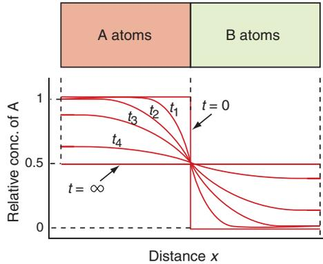
Figure 13.11 Intermixing by diffusion.
