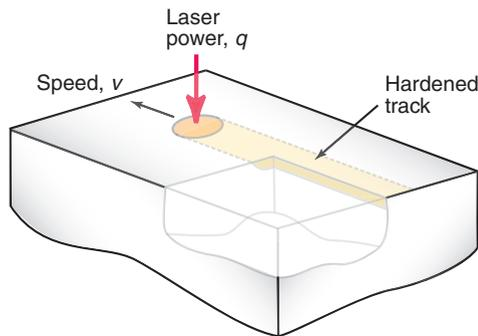
**Figure 19.10** Laser hardening: a surface treatment process that modifies microstructure. The traversing laser beam induces a rapid thermal cycle, causing phase changes on both heating and cooling. The track below the path of the laser has a different final microstructure of high hardness.
