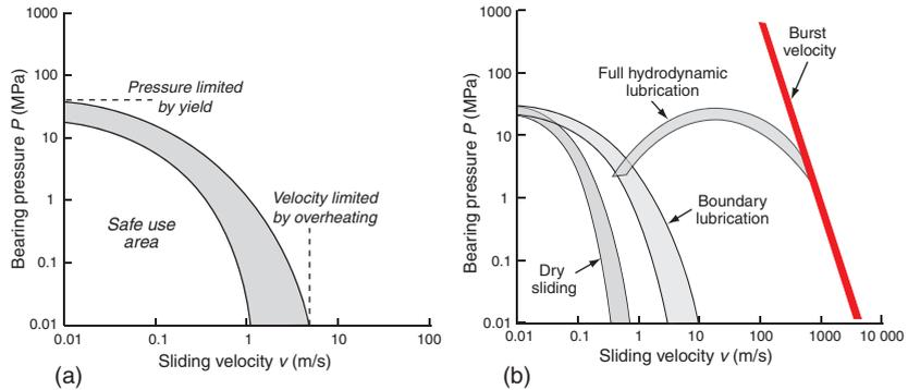
**Figure 11.11** (a) A  $P$ - $v$  curve for a bearing material. (b)  $P$ - $v$  envelopes for various lubricated and unlubricated sliding, ultimately limited by the disintegration of the bearing under centrifugal force at very high velocities.
