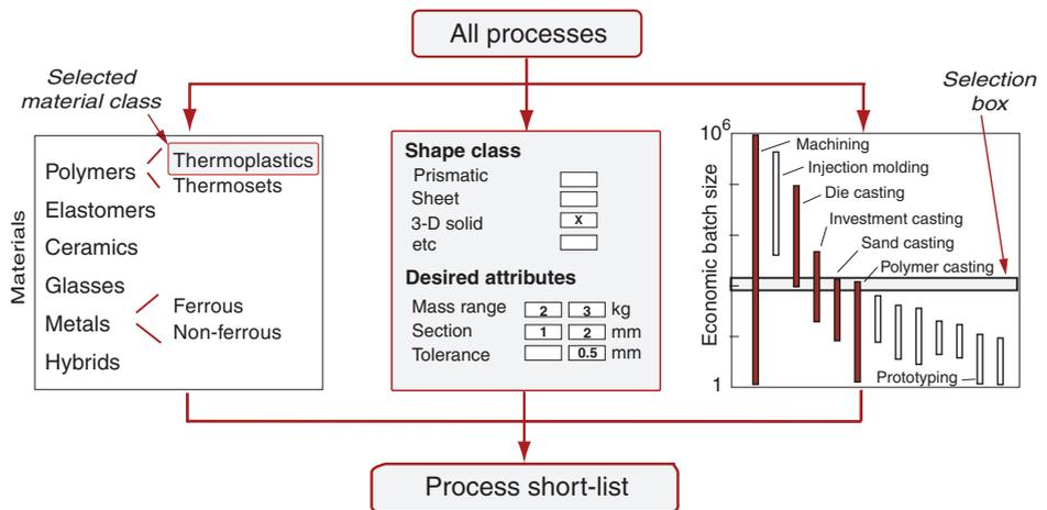
**Figure 18.18** Schematic of the screening steps in selecting process (here for shaping). First specify classes such as material and shape; then screen on numeric attributes, plotted graphically to the right as bar charts. In the CES software, target design requirements can also be entered through dialog boxes, shown in the center.
