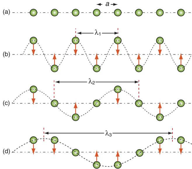
**Figure 12.8** Thermal energy involves atom vibrations. There is one longitudinal mode of vibration and two transverse modes, one of which is shown here. The shortest meaningful wavelength,  $\lambda_1 = 2a$ , is shown in (b).
