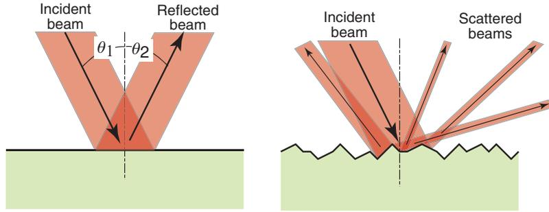
**Figure 16.2** Optically flat, reflective surfaces give specular reflection, such that  $\theta_1 = \theta_2$ . The angles of incidence and reflection are always equal, but the rough surface gives diffuse reflection even though the angles of incidence and reflection are still, locally, equal.
