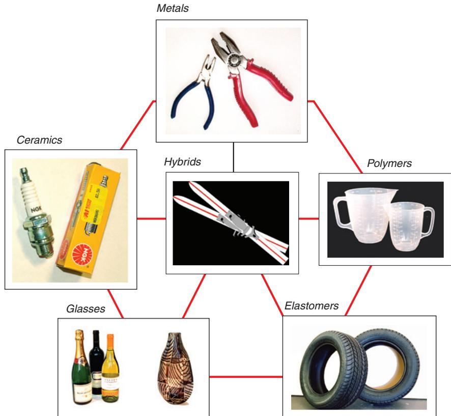
**Figure 2.2** Examples of each material family. The arrangement follows the general pattern of Figure 2.1. The central hybrid here is a sandwich structure made by combining stiff, strong face sheets of aluminum with a low-density core of balsa wood.
