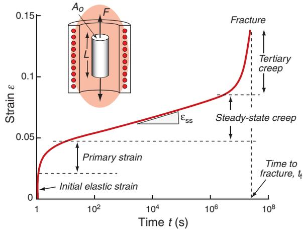
Figure 13.3 Creep testing and the creep curve, showing how strain  $\epsilon$  increases with time  $t$  up to the fracture time  $t_f$ .
