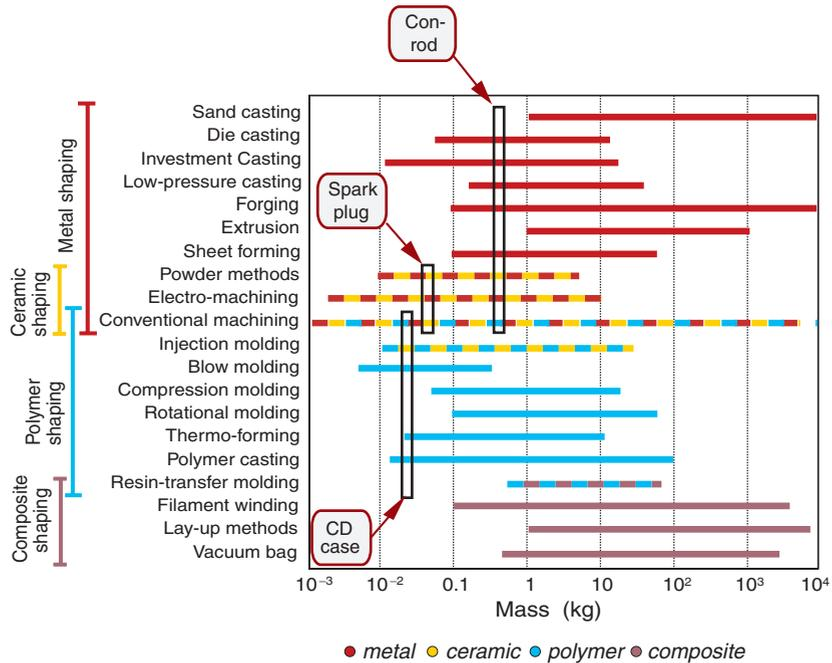
**Figure 18.3** The process–mass range bar chart for shaping processes. Ignore, on first reading, the boxes; they refer to case studies to come. The colors refer to the material, as in Figure 18.2. Multiple colors indicate compatibility with more than one family.
