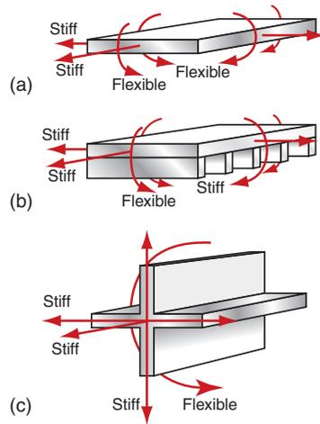
**Figure 5.19** The flexural degrees of freedom of three alternative section shapes. (a) Thin plates are flexible about any axis in the plane of the plate, but are otherwise stiff. (b) Ribbed plates are flexible about one in-plane axis but not in others. (c) Cruciform beams are stiff in bending but can be twisted easily.
