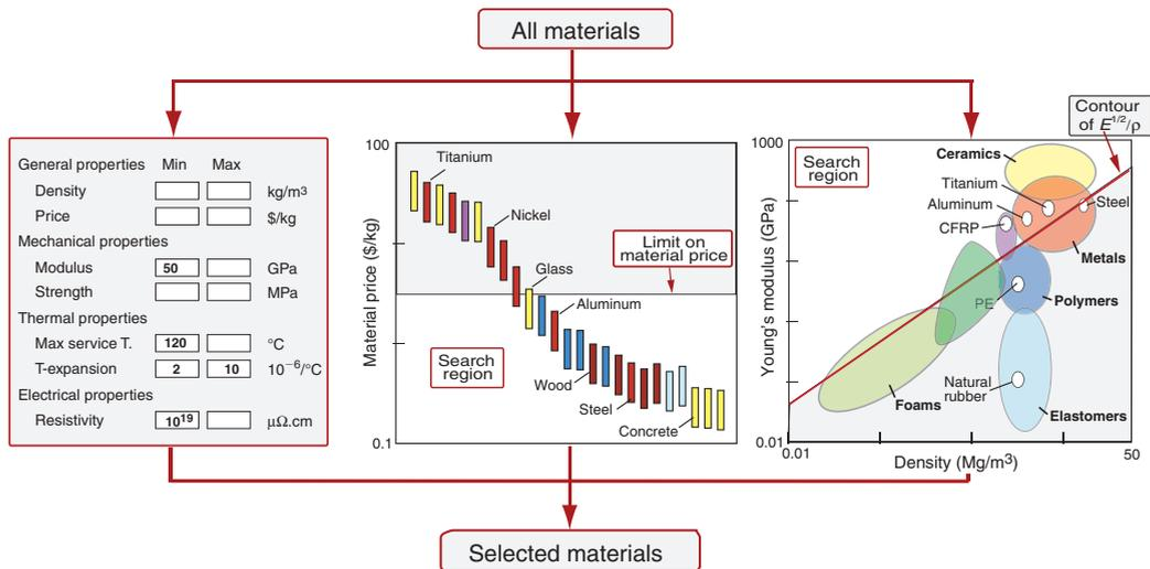
**Figure 5.12** Computer-aided selection using the CES software. The schematic shows the three types of selection window. They can be used in any order and any combination. The selection engine isolates the subset of materials that pass all the selection stages.
