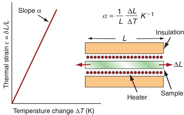
**Figure 12.2** Measuring the thermal expansion coefficient,  $\alpha$ . Its units are  $1/\text{K}$  or, more usually,  $10^{-6}/\text{K}$  (microstrain/ $\text{K}$ ).
