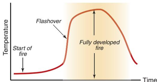
Figure 17.4 The temperature rise during a fire.
