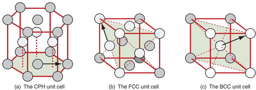
**Figure 4.11** Unit cells. All the atoms are of the same type, but are shaded differently to emphasize their positions. (a) The close-packed hexagonal (CPH) structure. (b) The close-packed face-centered cubic (FCC) structure. (c) The non-close-packed body-centered cubic (BCC) structure. Arrows show nearest neighbors.
