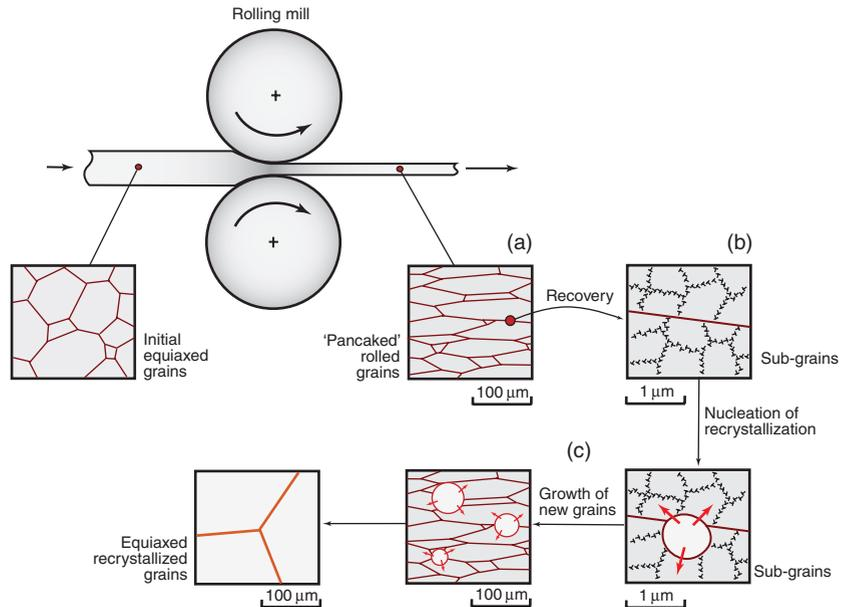
**Figure 19.6** Grain structure evolution in the solid state by deformation and annealing. (a) Grains pancake, following the change in shape of the component. (b) The recovery mechanism: dislocations rearrange as sub-grains (shown on a large scale). (c) The recrystallization mechanism: new grains form by migration of boundaries from a few sub-grain nuclei, wiping out the dislocations in the deformed microstructure.
