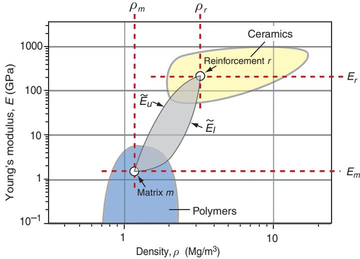
**Figure 4.22** Composites made from a matrix  $m$  with a reinforcement  $r$  have moduli and densities, depending on the volume fraction and form of the reinforcement, that lie within the gray shaded lozenge bracketed by equations (4.21) and (4.22). Here the matrix is a polymer and the reinforcement a ceramic, but the same argument holds for any combination.
