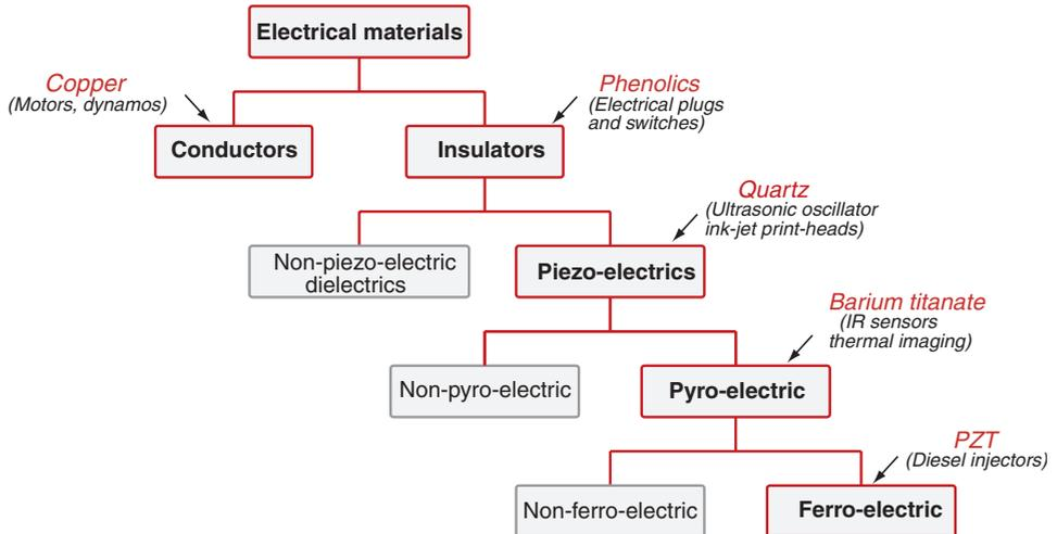
Figure 14.1 The hierarchy of electrical behavior. The interesting ones are boxed in red, with examples of materials and applications. Their nature and origins are described in this chapter.
