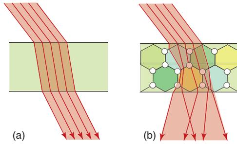
**Figure 16.10** (a) A pure glass with no internal structure and a wide band gap is completely transparent. (b) Light entering a polycrystalline ceramic or a partly crystalline polymer suffers multiple refraction and is also scattered by porosity, making it translucent.
