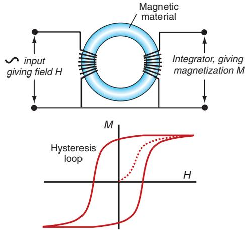
Figure 15.6 Measuring the hysteresis curve.
