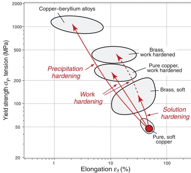
**Figure 6.21** Strengthening mechanisms and the consequent drop in ductility, here shown for copper alloys. The mechanisms are frequently combined. The greater the strength, the lower the ductility (the elongation to fracture,  $\epsilon_f$ ).
