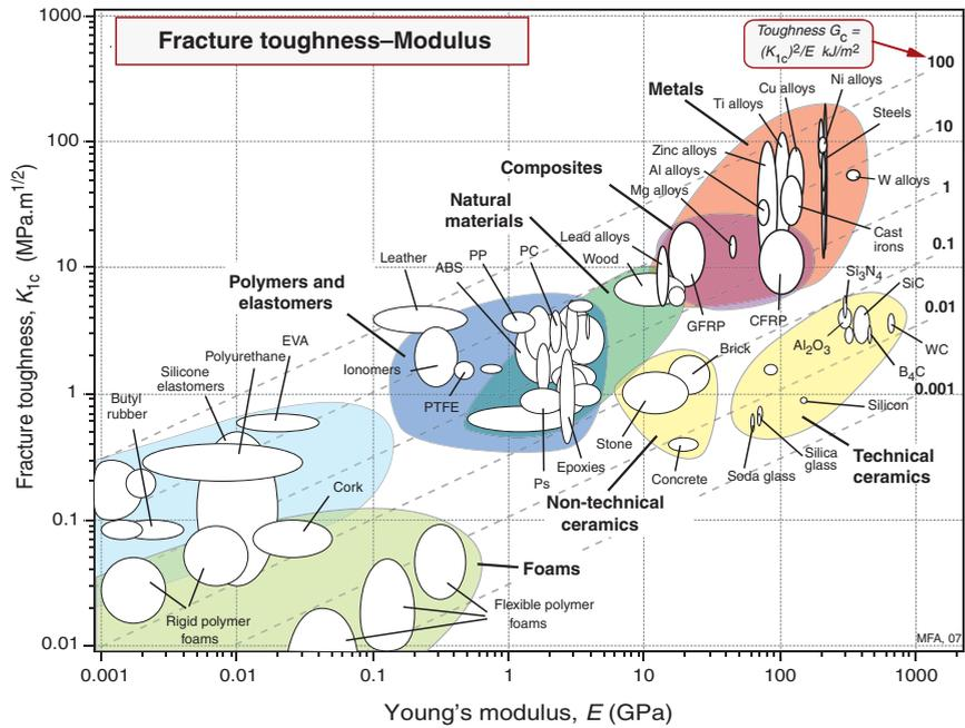
Figure 8.8 A chart of fracture toughness  $K_{Ic}$  and modulus  $E$ . The contours show the toughness,  $G_c$ .
