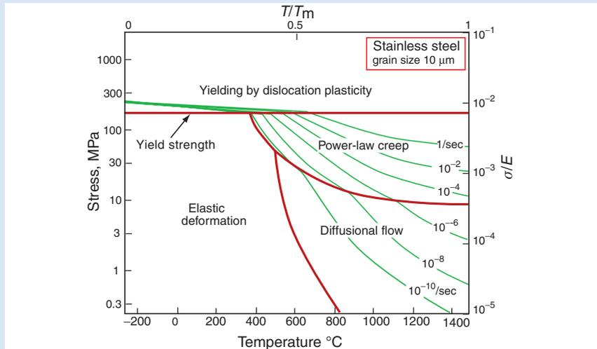
**Exercise E13.8** A stainless steel suspension cable in a furnace is subjected to a stress of 100 MPa at 700°C. Its creep rate is found to be unacceptably high. By what mechanism is creep occurring? What action would you suggest to tackle the problem? The figure shows the deformation mechanism map for the material.
