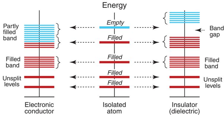
**Figure 14.9** Conductors, on the left, have a partly filled outer band—electrons in it can move easily. Insulators, on the right, have an outer filled band, separated from the nearest unfilled band by a band gap. (Red bands are filled, blue bands are empty.)
