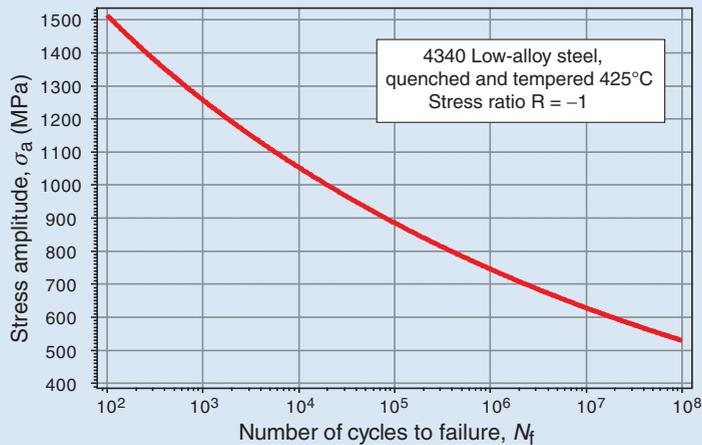
**Exercise E10.7** The component of the previous exercise was made and tested. It failed in less than  $10^5$  cycles. A post-mortem revealed that it had fractured at the root of a threaded end, shown in (b) in the figure. The threads have a depth of 1.5 mm and a root radius of 0.2 mm. Given this additional information, how many cycles would you expect it to survive?
