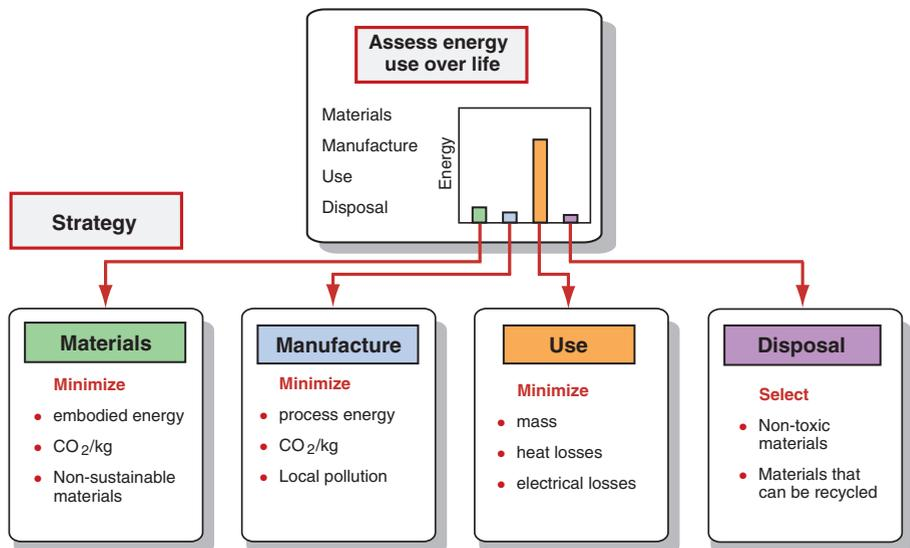
**Figure 20.12** Rational use of the database starts with an analysis of the phase of life to be targeted. The decision then guides the method of selection to minimize the impact of the phase on the environment.
