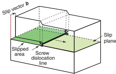
Figure 6.13 A screw dislocation. The slip vector  $\mathbf{b}$  is parallel to the dislocation line  $\mathbf{S}\text{--}\mathbf{S}$ .
