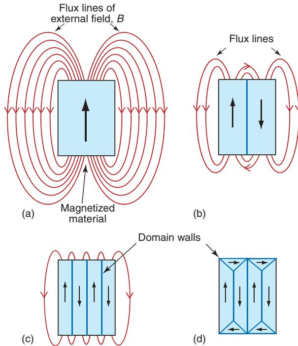
**Figure 15.12** Domains allow a compromise: the cancellation of the external field while retaining magnetization of the material itself. The arrows show the direction of magnetization.
