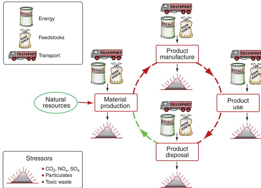
**Figure 20.3** The material life cycle. Ore and feedstock are mined and processed to yield a material. This is manufactured into a product that is used and, at the end of its life, discarded or recycled. Energy and materials are consumed in each phase, generating waste heat and solid, liquid and gaseous emissions.
