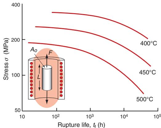
Figure 13.5 Creep fracture times. The scales are logarithmic. The data are typical of carbon steel.
