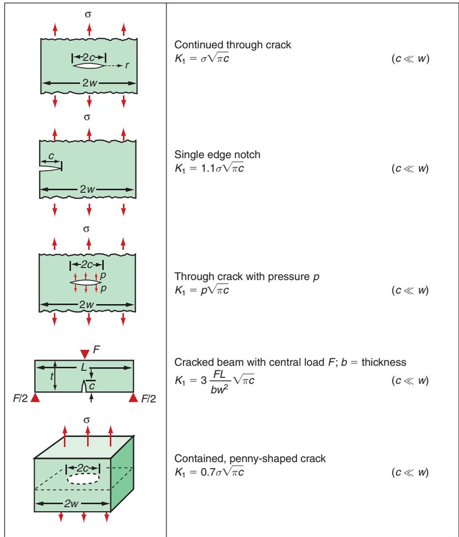
Figure 10.2 Stress intensities  $K_1$  associated with short cracks.
