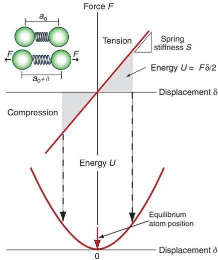
**Figure 4.19** Atoms in crystals and glasses are linked by atomic bonds that behave like springs. The bond stiffness is  $S = F/\delta$ . Stretching or compressing the bond by a displacement  $\delta$  stores energy  $U = F\delta/2$ . The equilibrium (no force) atom separation is at the bottom of the energy well.
