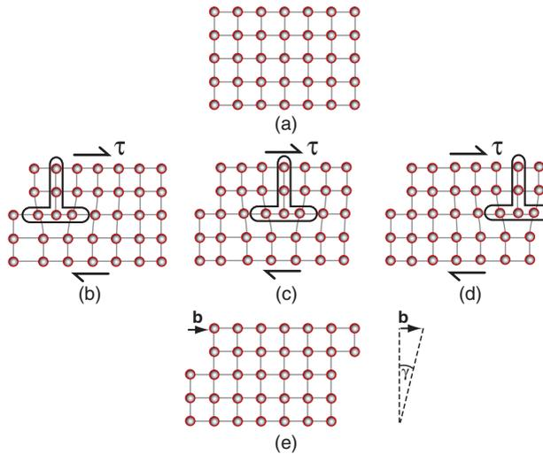
**Figure 6.12** An initially perfect crystal is shown in (a). The passage of the dislocation across the slip plan, shown in the sequence (b), (c) and (d), shears the upper part of the crystal over the lower part by the slip vector  $b$ . When it leaves the crystal has suffered a shear strain  $\gamma$ .
