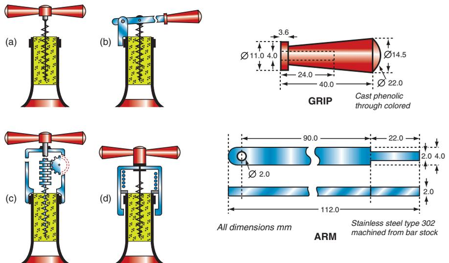
**Figure 3.3** Embodiment sketches for the first concept: direct pull, levered pull, geared pull and spring-assisted pull. Each system is made up of components that perform a sub-function. Detailed design drawings for the lever of embodiment (b) are shown on the right.
