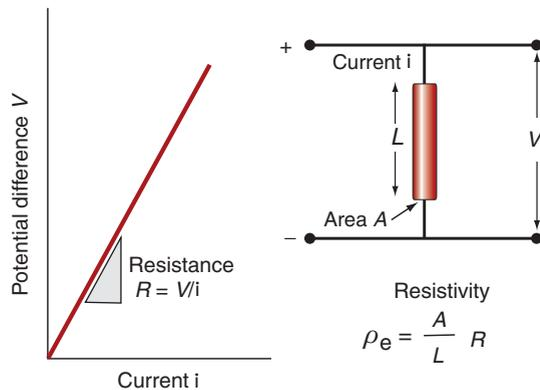
Figure 14.2 Electrical resistivity,  $\rho_e$ . Its value ranges from 1 to  $10^{24} \mu\Omega \cdot \text{cm}$ .
