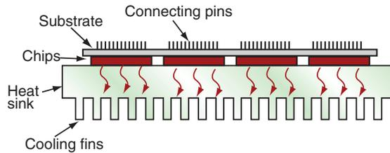
Figure 14.21 A heat sink. It must conduct heat but not electricity.
