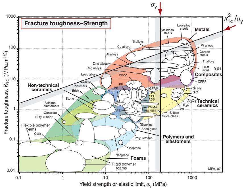
**Figure 10.6** Selecting the best materials for leak-before-break design. The additional requirement of high yield strength is also shown. The best choices are the materials in the small area at the top right.
