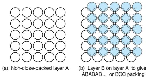
**Figure 4.9** (a) A square grid of spheres; it is a less efficient packing than that of the previous figure. (b) A second layer, B, nesting in the first, A; repeating this sequence gives ABAB... packing. If the sphere spacing is adjusted so that the gray spheres lie on the corners of a cube, the result is the non-close-packed BCC structure.
