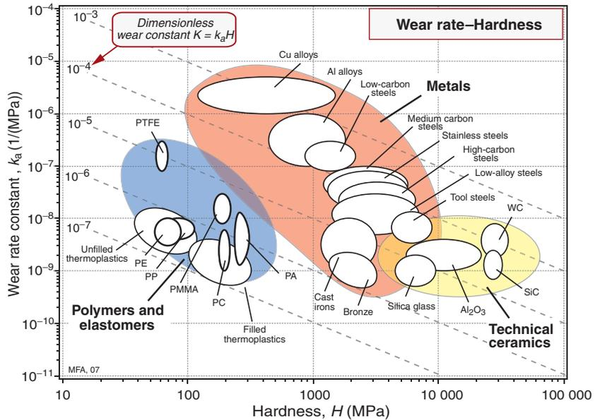
**Figure 11.3** The normalized wear rate for lubricated sliding,  $k_a$  plotted against hardness  $H$ , here expressed in MPa rather than Vickers ( $H$  in MPa =  $10 H_v$ ). The chart gives an overview of the way in which common engineering materials behave.
