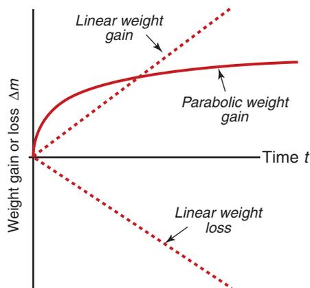
Figure 17.2 Oxidation rates: linear weight gain, parabolic gain and linear loss.
