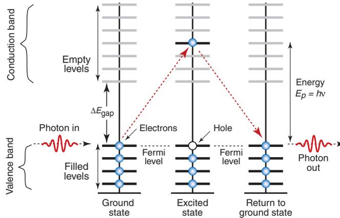
**Figure 16.9** Dielectrics have a full band, separated from the empty conduction band by an energy gap. The material cannot capture photons with energy less than  $\Delta E_{\text{gap}}$ , meaning that, for those frequencies, the material is transparent. Photons with energy greater than  $\Delta E_{\text{gap}}$  are absorbed, as illustrated here.
