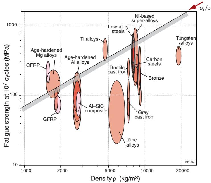
Figure 10.8 Endurance limit and density for high-strength metals and composites. (All materials with  $K_{1c} < 15 \text{ MPa}\cdot\text{m}^{1/2}$  were screened out before making this chart.)
