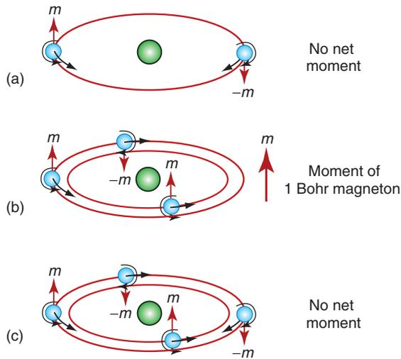
**Figure 15.10** Orbital and electron spins create a magnetic dipole. Even numbers of electrons filling energy levels in pairs have moments that cancel, as in (a) and (c). An unpaired electron gives the atom a permanent magnetic moment, as in (b).
