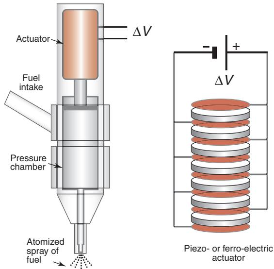
**Figure 14.25** A diesel injector. The actuator of the injector must be very precise to meter the fuel accurately, and must adapt its timing and stroke to match the conditions of the engine. Piezo- or ferro-electric stacks, like that shown on the right, offer the best control.
