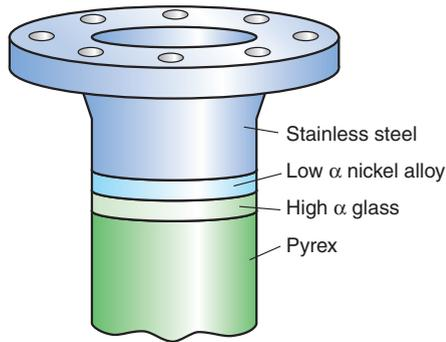
**Figure 12.13** A graded joint. The high expansion stainless steel is bonded to a nickel alloy of lower expansion, the low expansion Pyrex (a borosilicate glass) is bonded to a glass with higher expansion, and the set are assembled to give a stepwise graded expansion joint.
