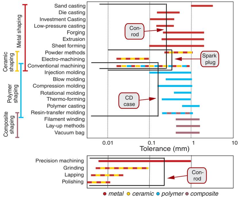
**Figure 18.11** The process—tolerance bar chart for shaping processes and some finishing processes, enabling process chains to be selected. The chart is color coded by material and annotated with the target values for the case studies.
