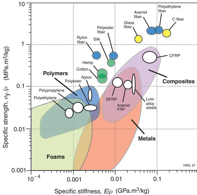
**Figure 19.14** Specific strength—specific modulus property chart. Bulk polymers are stiffened and strengthened by drawing into fibres, competing with natural, carbon and glass fibres. Most products use the fibres in a composite, such as CFRP, or woven into a fabric.
