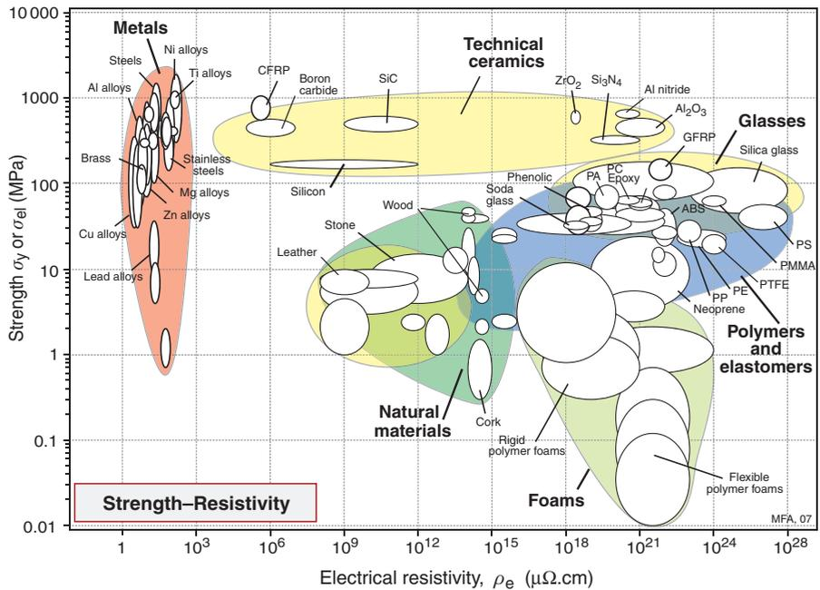
Figure 14.6 Material property chart for electrical resistivity  $\rho_e$  and yield strength  $\sigma_y$  or elastic limit  $\sigma_{el}$ .
