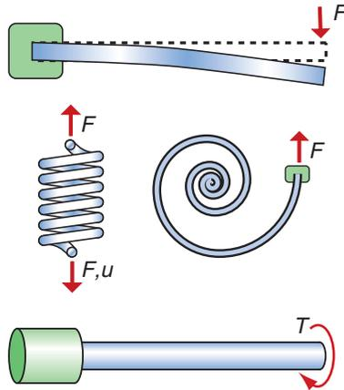
**Figure 7.10** Springs: leaf, helical, spiral and torsion bar. Springs store energy. The best material for a spring, regardless of its shape or the way it is loaded, is that of a material with a large value of  $\sigma_y^2/E$ .
