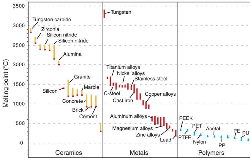
Figure 13.6 Melting points of ceramics, metals and polymers.
