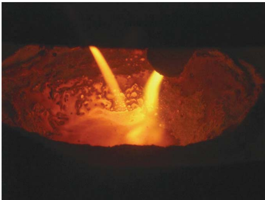
Fig. 11.3 Photo of plasma torches melting glass batch
