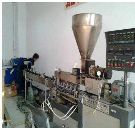
Figure 1. Double screw extruder.
